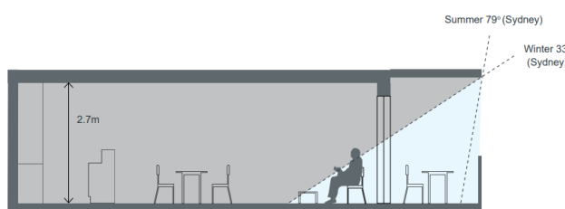
Figure 4A.2 Shading devices on balconies should shade summer sun and allow winter sun access to living areas
