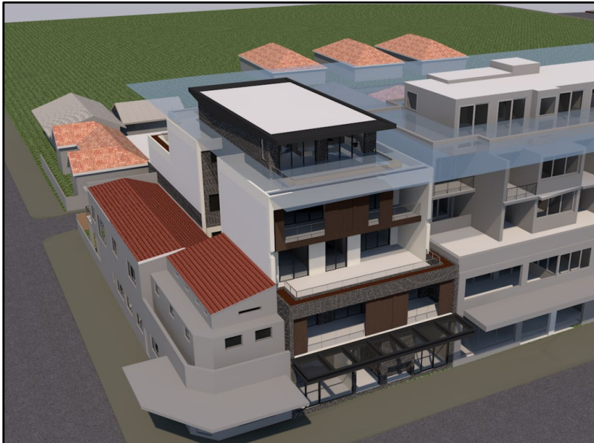
Figure 5: Height plane diagram demonstrating the portions of the development that site above the height standard of 14m. The proposed height is compatible with the adjoining southern neighbour at No. 1027-1043, which exceeds the height standard in a similar way
